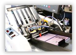
Designed to handle most gluing and folding jobs for 11 x 17 inch sheets and smaller
